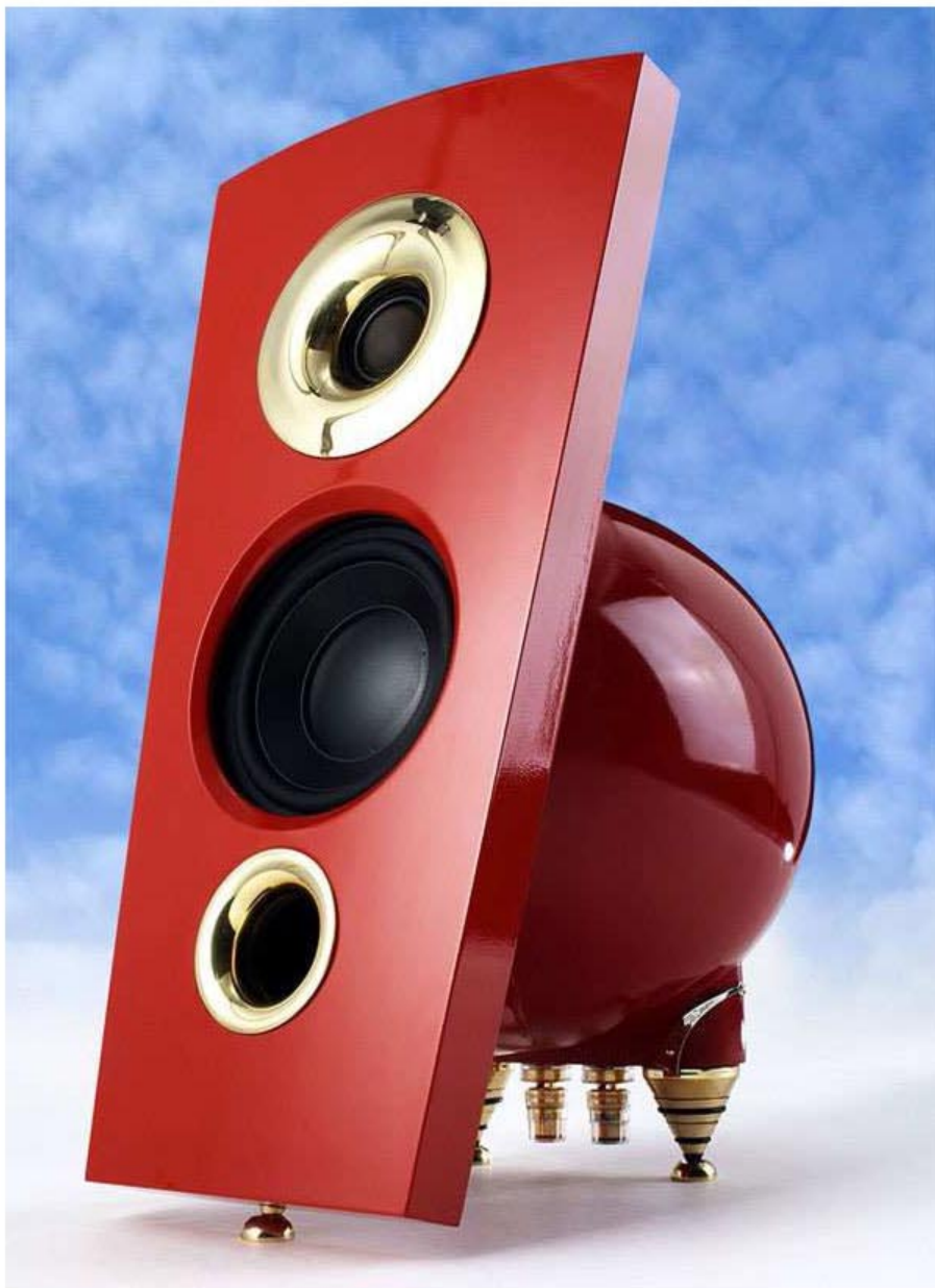
None of EBTB's speakers are large, including the flagship Terra II, which stands only 15 inches tall. This 2-way design employs a 1-inch silk-dome tweeter and 4-inch, front-ported midbass driver to achieve a frequency response from 69Hz to 25kHz ( \pm 3\text{dB} ) for a list price of $1949 each.
